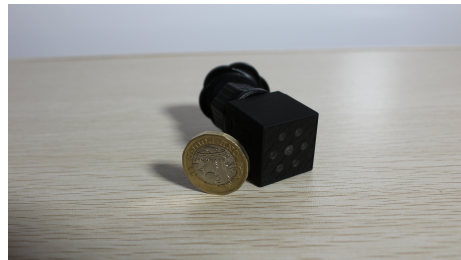
FIGURE 2.25: A small-form-factor magnetic surveillance camera, of the type that might be used in shoulder-surfing attacks aided by recording devices. UK pound coin shown for scale. Photograph by author.
