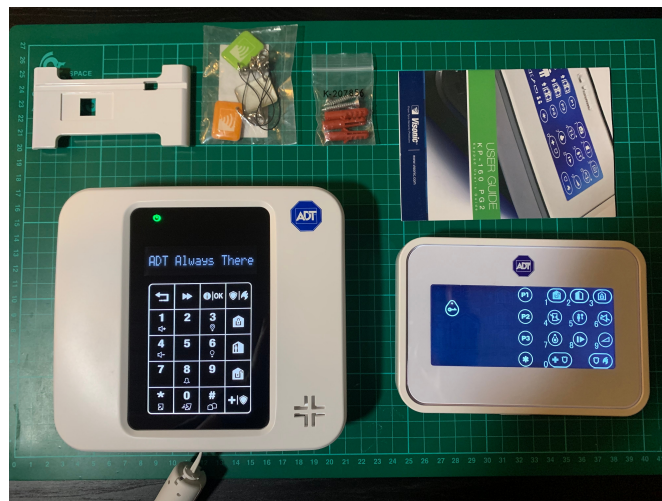
FIGURE 2.36: An ADT branded Visonic PowerMaster PM-360R central control panel (bottom left) with enrolled KP-160 PG2 keypad (bottom-right). Also pictured: tamper-resistant back panel for KP-160 PG2 (top left), bundled Visonic “Chicklet” K-303465 Proximity Tags (second from top left), bundled wall fixings (top centre) and instruction manual for the KP-160 PG2 (top right).
