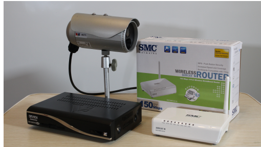
FIGURE 2.7: A selection of devices made based on data in (Antonakakis et al., 2017) that are potentially vulnerable to infection by Mirai . From left: Dreambox DM500V8 Multimedia Receiver, ACTi D32 Security Camera, SMC Barricade Wireless Broadband Router. Photograph by author.
