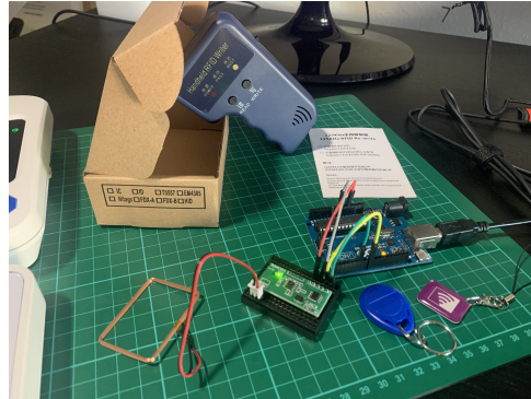
FIGURE 2.40: Equipment set up for cloning of the purple Visonic proximity tag (foreground) by the blue EM4100 tag duplicator (background) to the rewritable generic blue EM4100-compatible RFID key fob (foreground). After cloning, its memory array is identical to that of the Visonic proximity tag, shown in Figure 2.39b. For factory programming of the generic tag, see appendix Figure 2.40. Photograph by author.
