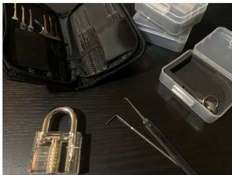
FIGURE 2.35: A set of pin-tumbler lock-picks and selection of transparent acrylic practice locks. Photograph by author.
